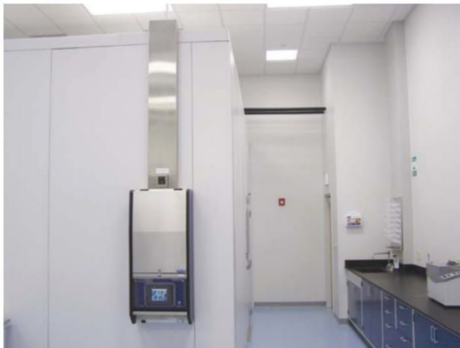
Fig. 14.2 ESI Walk-in stability chamber with CCS Touchscreen control ( Photo Courtesy of Metrics Inc. )
