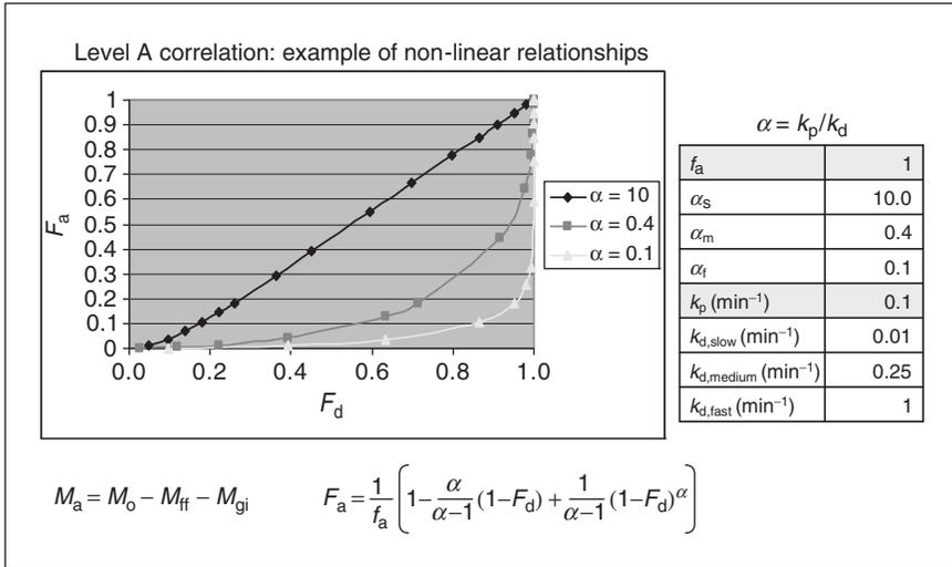
**Figure 4.3.13** Example of non-linear IVVC. Model of Polli *et al.* (1996). The model is based on the mass balance:  $M_o$  is the dose (initial amount of drug in the dosage form);  $M_{ff}$  the mass of drug remaining in the dosage form;  $M_{gi}$  the mass of drug in solution in the GI fluids;  $\alpha$  represents the ratio between the permeation rate constant ( $k_p$ ) and the dissolution rate constant ( $k_d$ ). For explanation see text.
