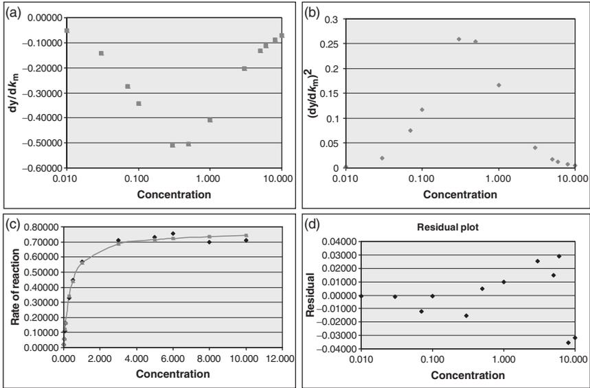
**Figure 4.3.15** (a) Derivate of the dependent variable with respect to the parameter ( $K_m$ ). (b) Squared value of the derivate in panel a. (c) plot of the dependent variable (rate of reaction) versus the independent one (substrate concentration). (d) Residual plot: differences between the experimental and the predicted values (residuals) versus concentration (independent variable). For explanation see text.
