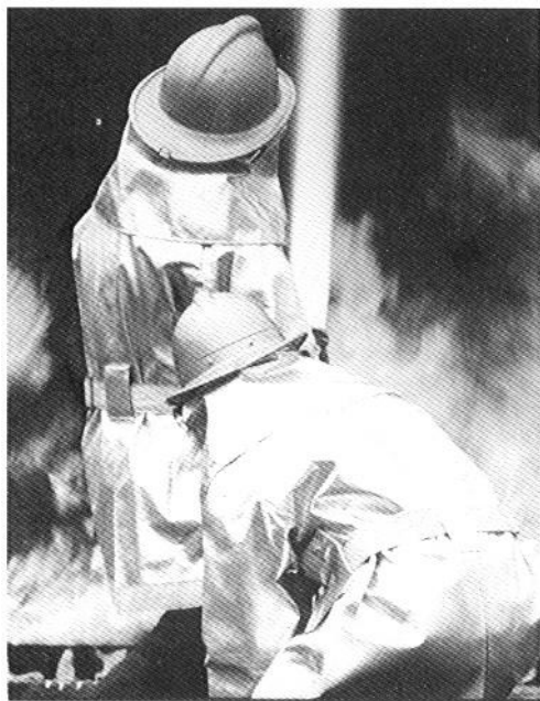
2.4 Firefighter uniform of meta -type aramid fiber (Du Pont, Japan).
