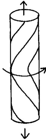
Fig. 18.2 — Untwisting under tension at a reversal point.
