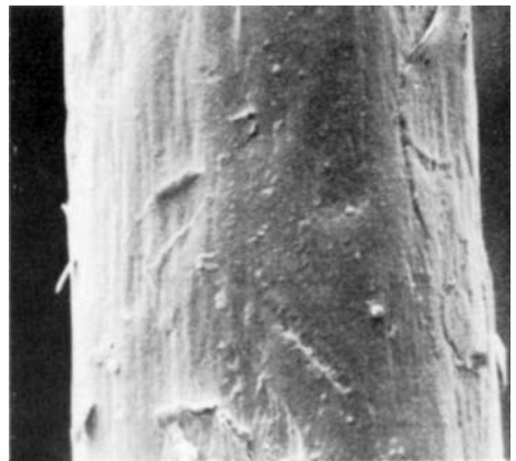
Plate 25B — Damage to abradant in testing of cotton fabrics: test details as in 25A.
