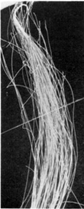
Plate 24D — Yarn-on-yarn abrasion testing, 1100 dtex industrial filament yarns, three wraps at wrap angle of 35°, 50 mm stroke, 52 cycles/min, in air at 65%, 20°C. (1), (2) Nylon, with tension weight of 200 g, failed at 35 000 cycles. (3), (4) Polyester, with tension weight of 800 g, failed at 2 cycles.
