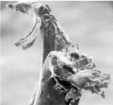
Plate24B — Tensile breakage of 77 dtex/16-filament nylon yarn, twisted to 100 turns/cm. (1) Broken yarn. (2)–(6) Individual filaments in broken ends.
