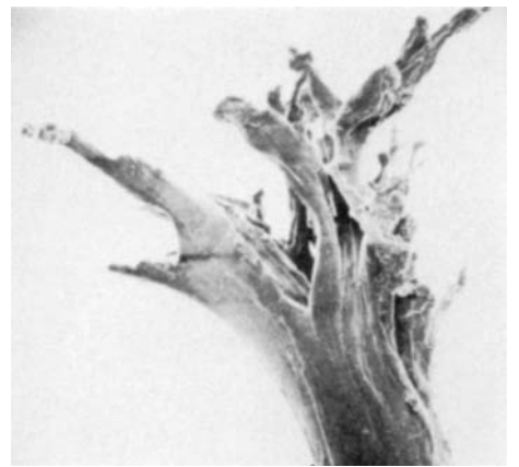
Plate24B — Tensile breakage of 77 dtex/16-filament nylon yarn, twisted to 100 turns/cm. (1) Broken yarn. (2)–(6) Individual filaments in broken ends.
