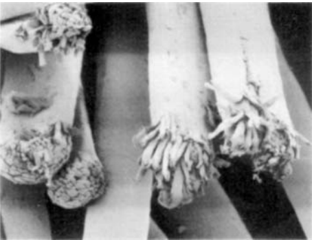
Plate 25M — Abrasion of woven wool/mohair fabric.
