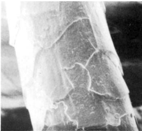
Plate 25B — Damage to abradant in testing of cotton fabrics: test details as in 25A.
