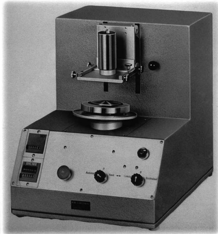
5.4 Karl Schroder Schopper Abrasion Testing Machine. Photograph supplied by SDL International and reproduced with kind permission.
