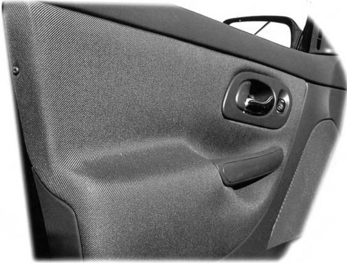
6.7 Integral door panel and arm rest.
