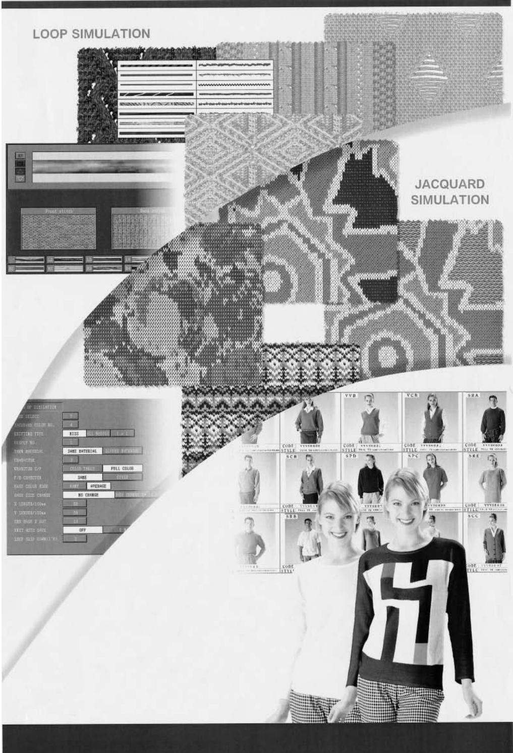
Fig. 12.3 The simulated knit package is mapped onto an image of a model to simulate the appearance of the final product. This image can also be used for evaluation and sales promotion purposes [Shima Seiki].
