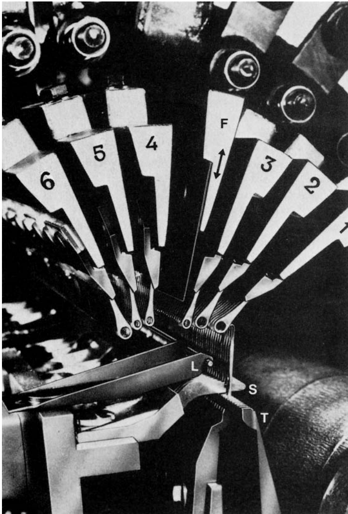
Fig. 27.2 Multi-purpose fall-plate raschel machine [Karl Mayer]. Bars 1, 2, 3 – fall-plate guide bars; bar 4 – knitting guide bar; bars 5, 6 – inlay guide bars. L = latch opening wire; S = holding-down sinker; T = trick plate; F = fall-plate.
