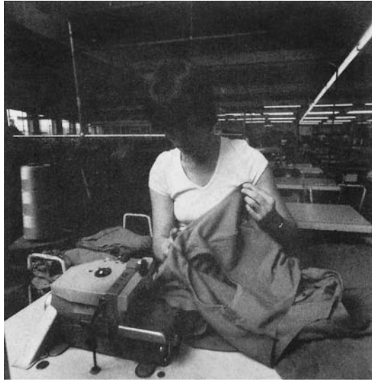
Fig. 6.3 Overlock seaming [Corah].
