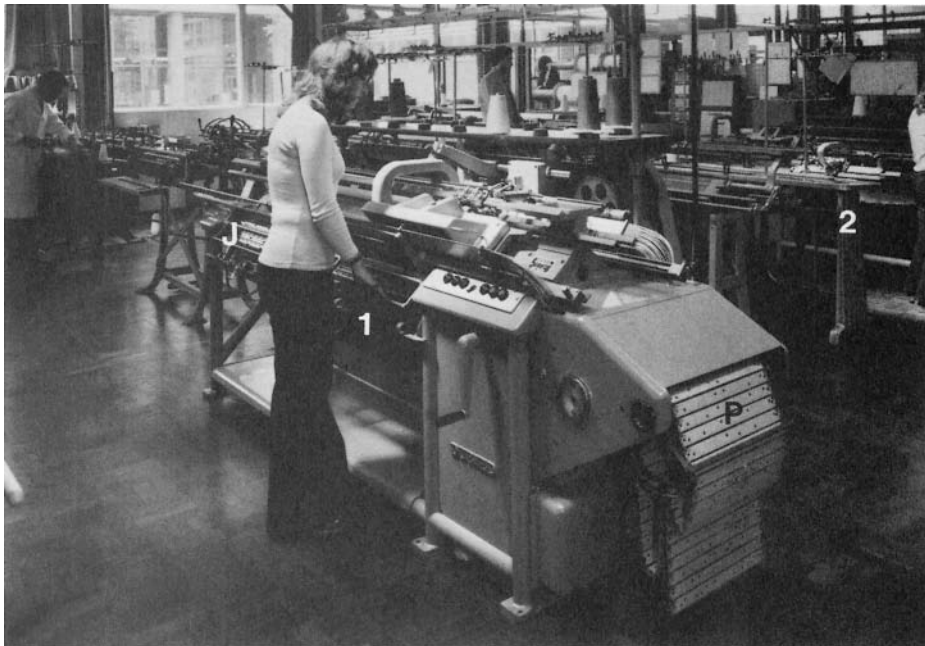
Fig. 8.2 Mechanically controlled flat knitting machines. 1 = jacquard power flat; 2 = hand flat; J = jacquard selection steels; P = paste board movement cards.
