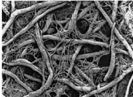
ACORDIS LYOCELL Fibrillation
