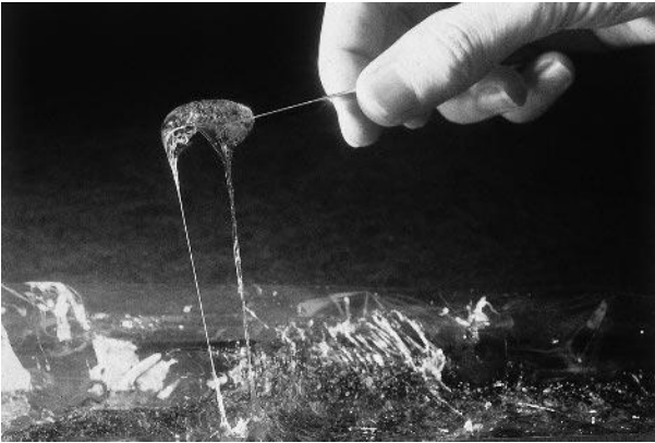
12 Cellulose in NMMO: fibre-forming potential evident.
