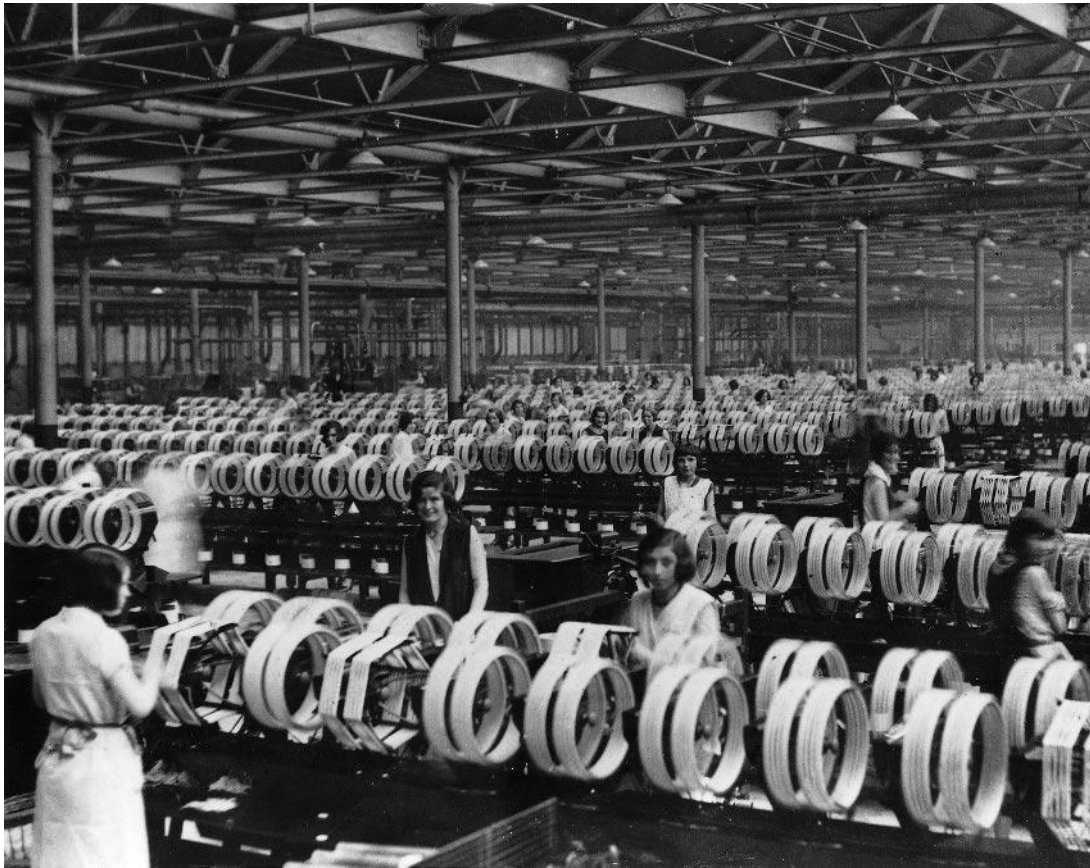
1 Viscose filament yarn process circa 1930: preparing hanks for washing.
