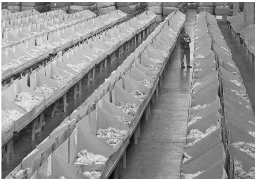
1.3 Photograph of a complete assembly of representative grab samples of New Zealand wool lots to be auctioned. Each numbered viewing box has a data sheet from a test-house and other information.
