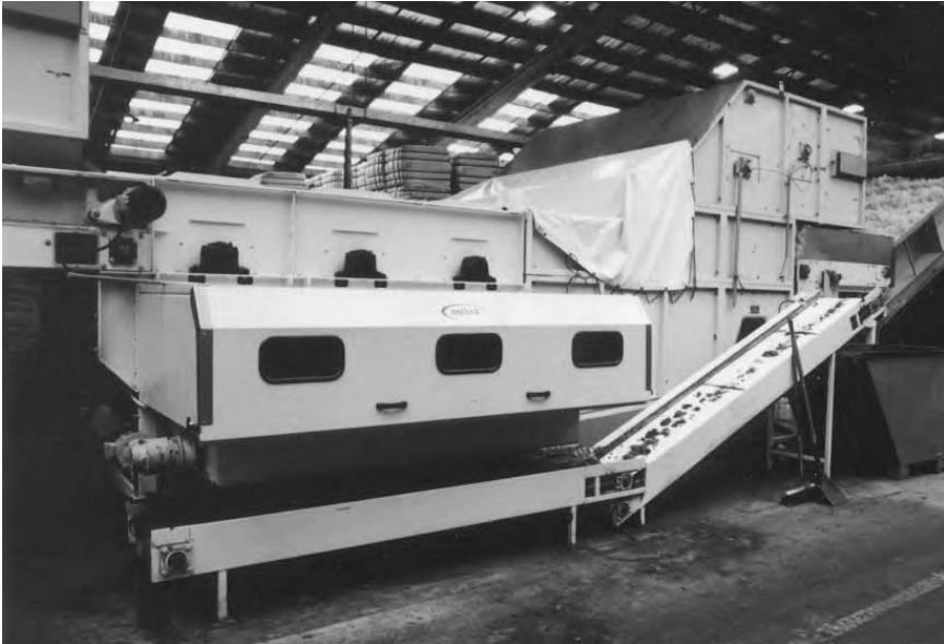
2.4 Three-drum greasy wool opener. [Courtesy of Kaputone Wool Scour (1994) Ltd.]
