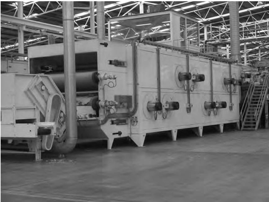
2.13 Modern sandwich-conveyor dryer. [Courtesy of Jandakot Wool Washing Pty Ltd.]
