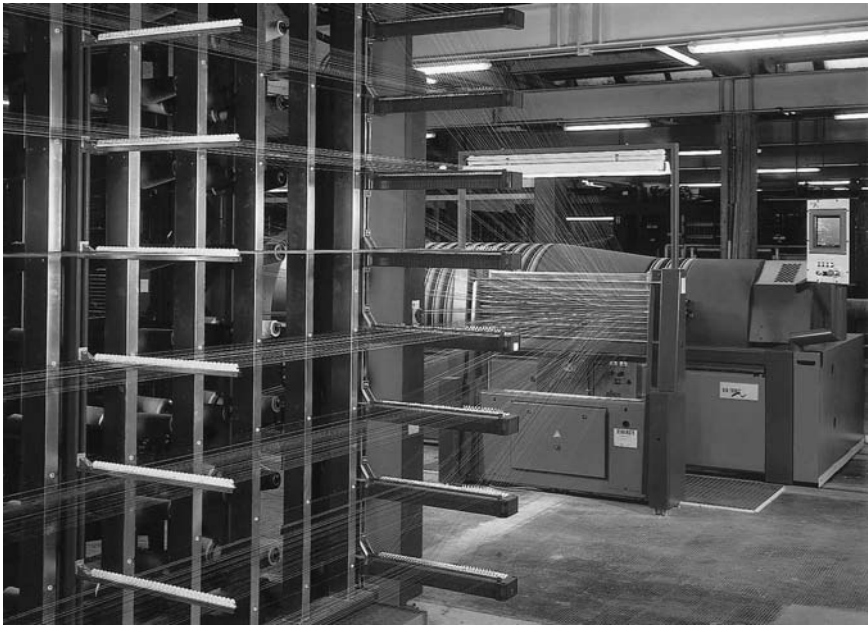
9.3 The Ben-tronic sectional warping machine and creel. [Source: Benninger. ]
