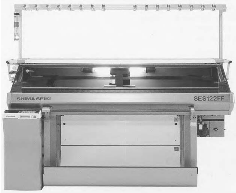
9.11 Flatbed knitting machine with computer control facility. [Source: Shima Seiko, Japan.]
