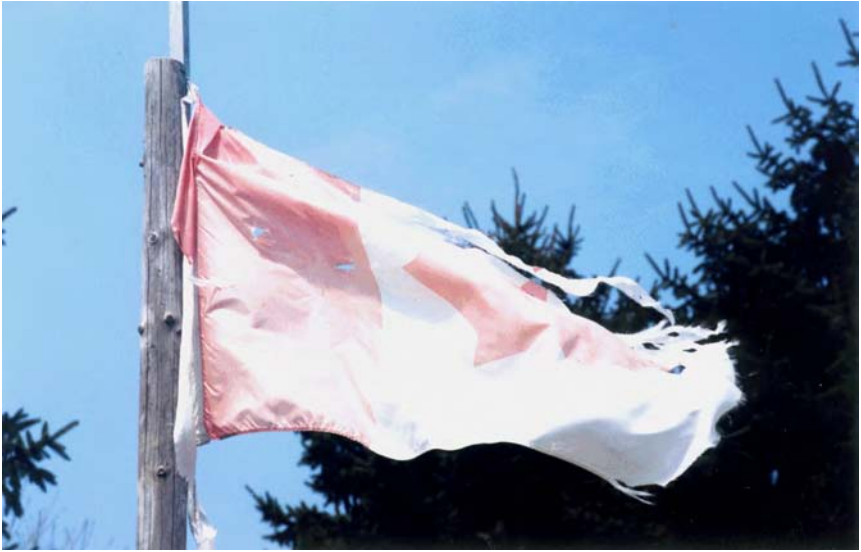
10.4 Effect of weathering on a nylon flag.
