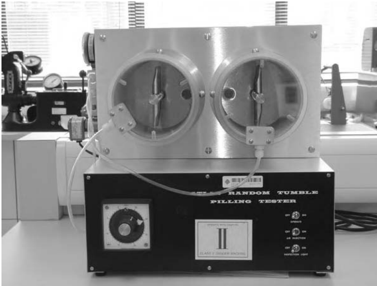
Figure 2.5 Random Tumble Pilling Tester.
