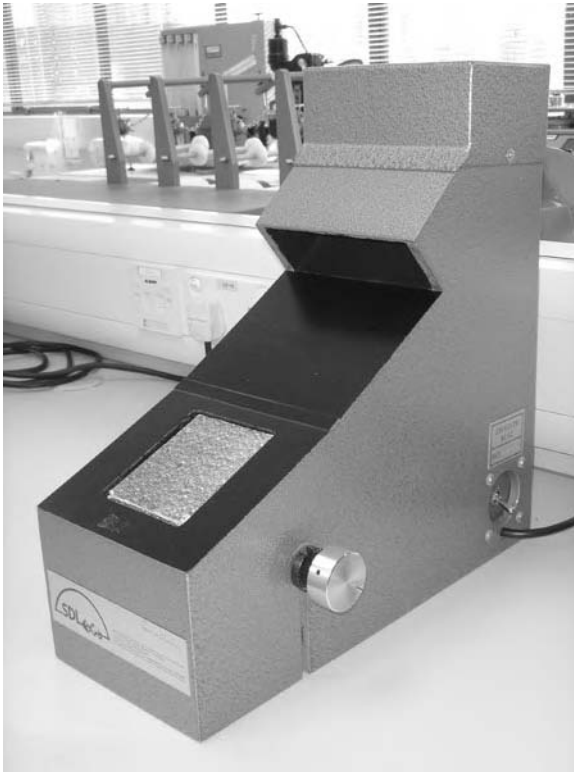
Figure 2.2 View device for pilling assessment.
