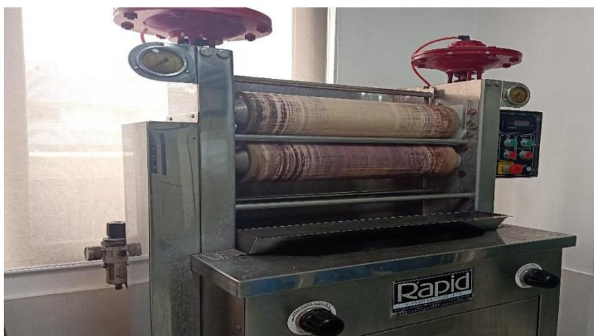
**Figure 1.** Cold pad batch lab dyeing machine
