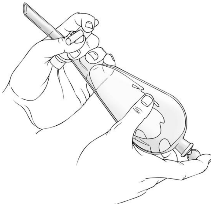
Figure 12.6 The correct way of shaking and venting a separatory funnel.
