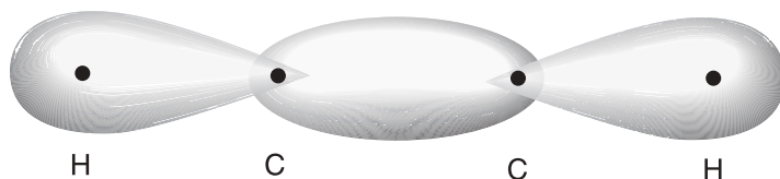
Fig. 1.6. The \sigma electrons of acetylene.
