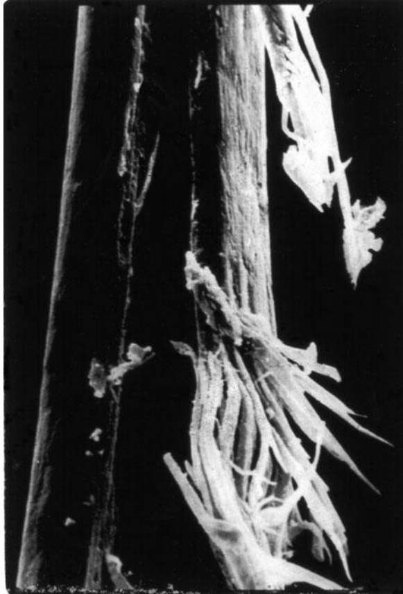
Fig. 1.30 SEM of a split hair. Note cortical cell fragments
