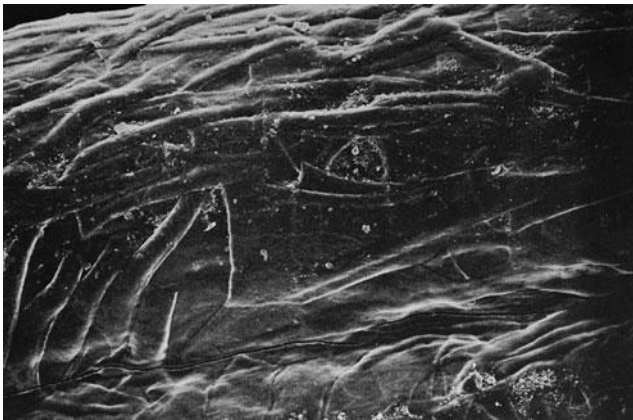
Fig. 5.10 Hair fiber exposed to ultraviolet radiation and then bleached for 15 min with alkaline peroxide. Note the decreased scale definition (SEM kindly provided by Sigrid Ruetsch)
