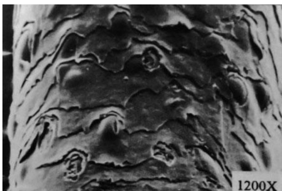
Fig. 6.35 Deep ovoidal cuticle cracks produced by thermal and extension cycling treatments by Garcia [149] (Reprinted with permission of the Journal of Cosmetic Science)
