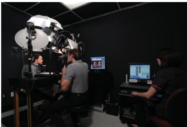
Figure 6.1 An example of a Stephens & Associates, Inc. photographic studio. The studio is equipped for taking photographs using standard lighting, parallel and polarized lighting, cross polarized lighting and raking light.
