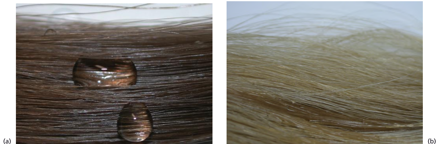
Figure 30.7 Change in surface hydrophobicity before (a) and after (b) bleaching.
