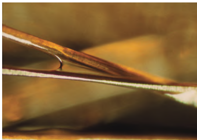
Figure 33.5 Hairspray bond – spot weld.
