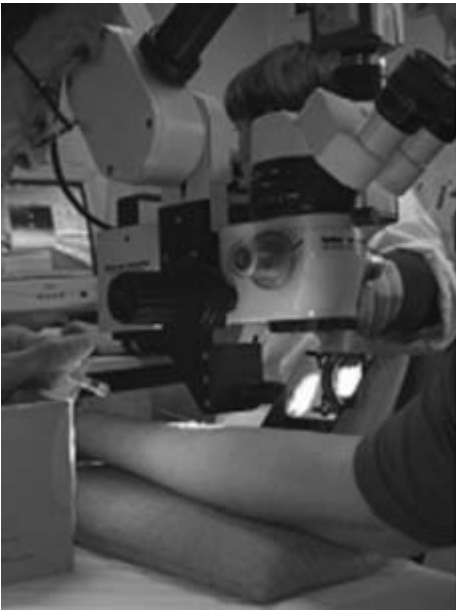
Figure 3 Contact angle visualization and measurement: tool rests on the use of a mirror directed 45^\circ to the skin “profile drop method.”
