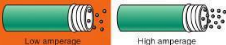
Figure 11-3 Amps measure the number of electrons flowing through the wire.
