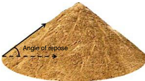
Figure 15.17 Angle of repose of a solid material. Source: Captain Sprite, https://commons.wikimedia.org/wiki/File:Angleofrepose.png . Used under CC BY-SA 2.5 https://creativecommons.org/licenses/by-sa/2.5/deed.en . © Wikipedia.
