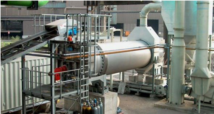
Figure 14.2 Rotary dryers. Source: Brookoffice, https://commons.wikimedia.org/wiki/File:Single_Shell_Rotary_Drum_Dryer.jpg . Used under CC BY-SA 3.0, http://creativecommons.org/licenses/by-sa/3.0 . © Wikipedia.
