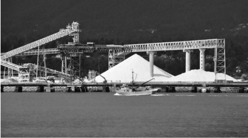
Figure 15.7 Belt conveyor for sulfur. Source: Leonard G, https://commons.wikimedia.org/wiki/File:AlbertaSulfurAtVancouverBC.jpg . Used under CC SA 1.0 https://creativecommons.org/licenses/sa/1.0/ . © Wikipedia.
