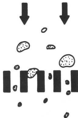
Figure 1.1. Filtration by surface straining (2) .
