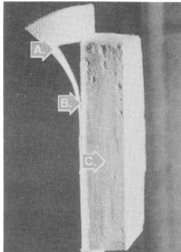
Figure 10.1. The three layers in precoat filtration: (A) a filter cloth or mesh, (B) the precoat layer protecting the cloth from plugging, (C) the filter cake.
