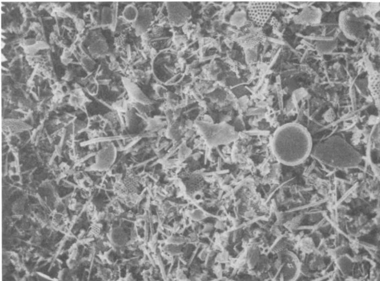
Figure 10.2. Diatomite filter aid at low magnification.
