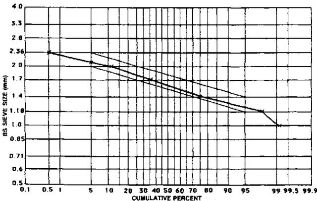
Figure 10.12. Example of a plot of sieve test data on a log/probability basis, with tramline limits (based on an example in British Water Standard<sup>(11)</sup>).
