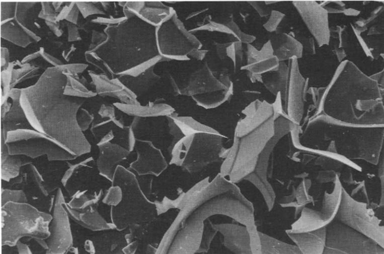
Figure 10.5. 'Harborlite 900S' expanded perlite at high magnification.
