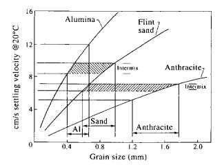
Figure 10.14. Settling velocity versus grain-size curves indicate the intermixing and layering of a threecomponent deep bed.
