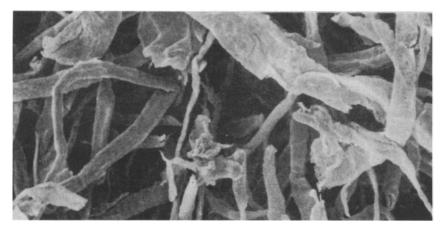
Figure 10.7. Celite 'Fibra-Cel SW-10' cellulose fibres at  $\times 200$  magnification.
