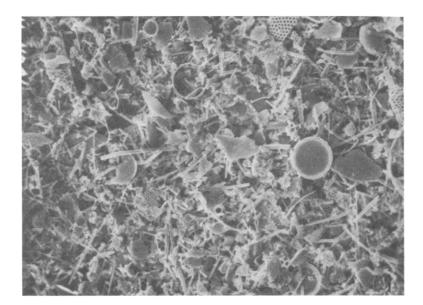
Figure 10.2. Diatomite filter aid at low magnification.
