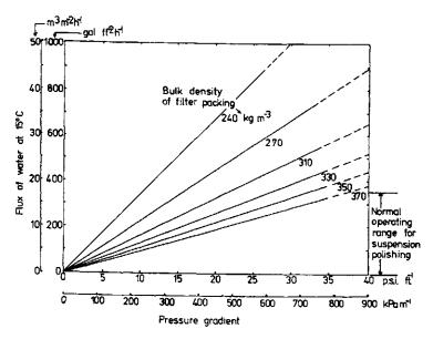
Figure 10.16. Flux versus pressure gradient of Howden-Wakeman filter.
