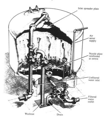
Figure 10.10. A vertical pressure sand filter.
