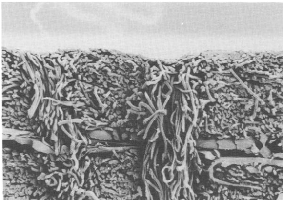
Figure 3.4. Cross section through a needle felt, showing the scrim and also the fibre re-orientation caused by the needling, at \times 62 magnification.
