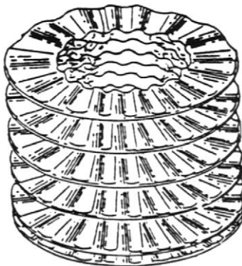
Figure 9.23. Schematic illustration of 3M Series 700B radial cartridge.
