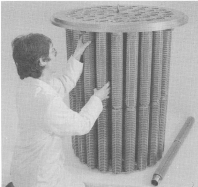
Figure 9.27. A multiple assembly of pleated sintered metal fibre cartridges for high temperature gas filtration.
