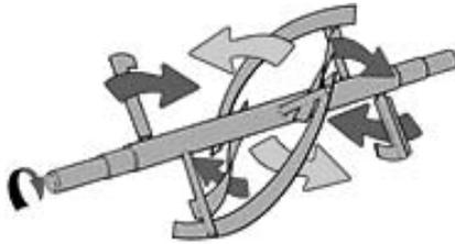
**Figure 15-41** Direction of solids movement in ribbon mixer. (Courtesy of Kemutec.)
