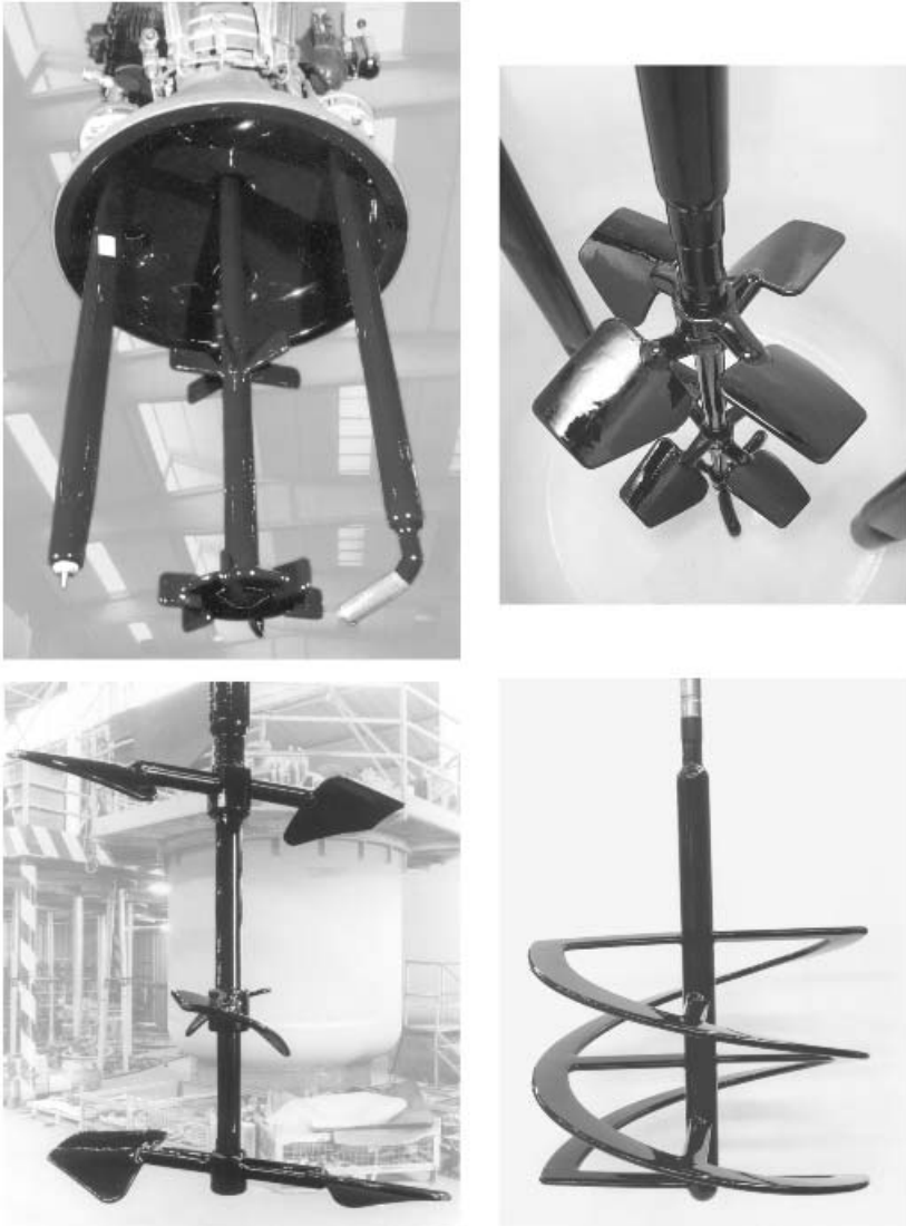
Figure 17-1 (c) ElcoLock ® and fixed impellers. (Courtesy of Tycon Technoglass, a Robbins & Myers company.)
