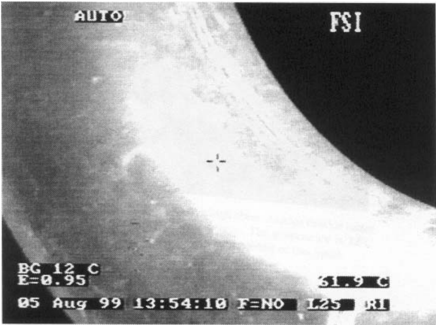
Figure 20-23 Thermograph of exit piping following a high-shear chlorine dioxide mixer in D_1 service. Elbow immediately following mixer discharge. The temperature is 12^\circ\text{C} higher along the top of the pipe. See insert for a color representation of this figure.
