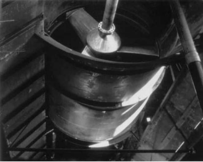
Figure 22-6 Full scale testing: a 3.2 m impeller in a 1 900 000 L test tank.
