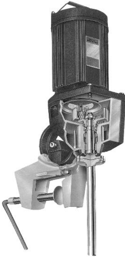
Figure 21-2 Gear-drive portable mixer. (Courtesy of Lightnin.)
