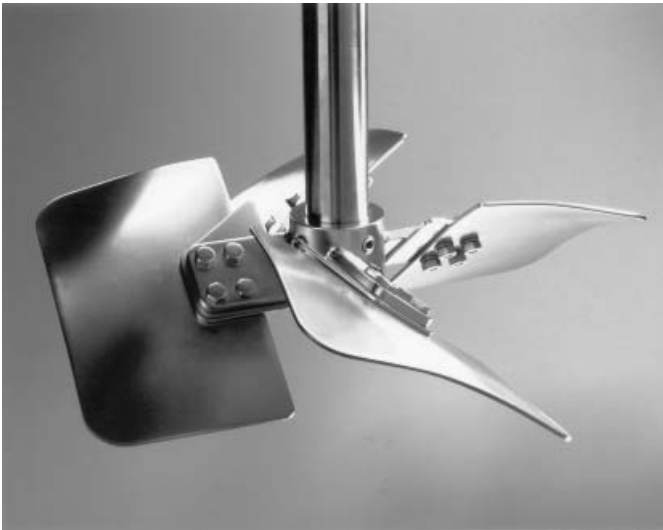
Figure 22-8 High solidity hydrofoil impeller for high viscosity or gas applications: N_p = 0.75 .
