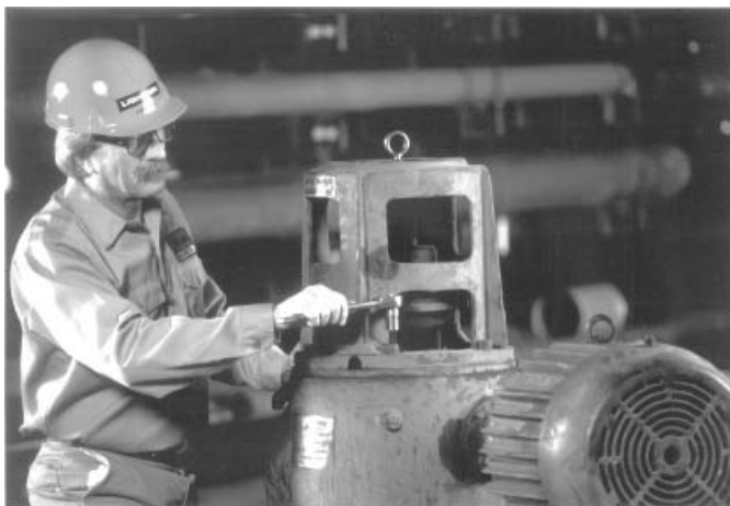
Figure 22-21 Service engineer adjusting speed reducer.
