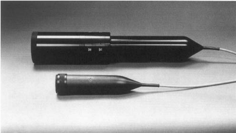
Figure 4-40 Modern commercial fiber optic-based LDA probes.
