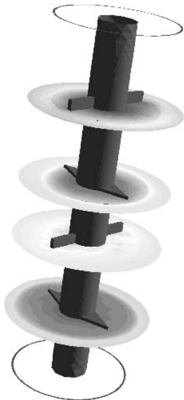
Figure 5-33 Contours of molecular weight distribution are used to assess the range of molecular weights in the product.
