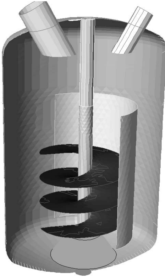
Figure 5-15 Geometry using solid surfaces with a cut in the wall and top to look inside.
