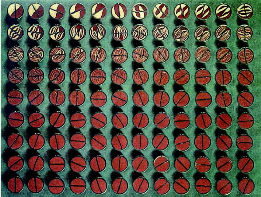
Figure 7-20 Laminar mixing of fluids by division and recombination (KMS mixer). Cross-sections of the mixer are shown in sequence from left to right, top to bottom. (Courtesy of Chemineer, Inc.)
