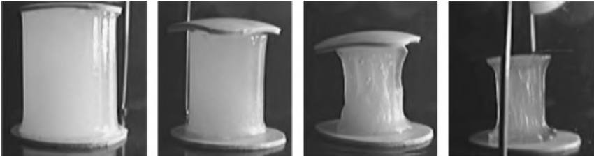
Fig. 5.15 Convective drying of a hydrogel (based on polyvinylpyrrolidone) (taken from Pakowski et al. (2006)).
