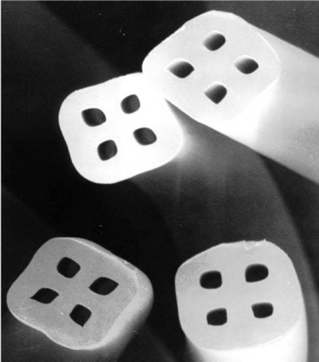
2.7 DuPont Antron ® carpet fibres in transverse cross-section (by courtesy of DuPont Commercial Flooring).
