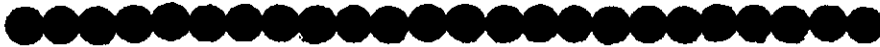
2.6 Cross-section of 24 threads side by side just touching in the space of one inch.
