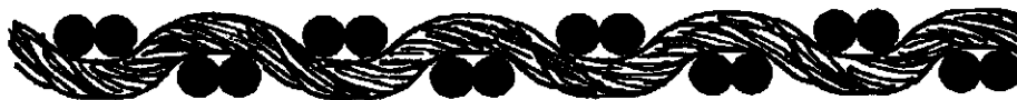
2.8 In 2/2 twill there is sufficient space to allow 16 threads in the space of one inch.
