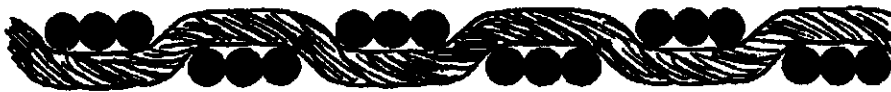
2.9 In 3/3 twill only six interlacings provides space for 18 threads in the space of one inch.
