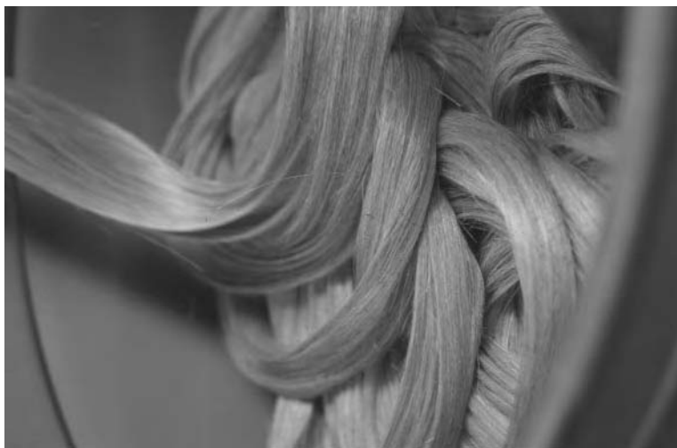
Figure 3.19 Line flax sliver being wound into 'can' after hackling. Source: Masters of Linen.
