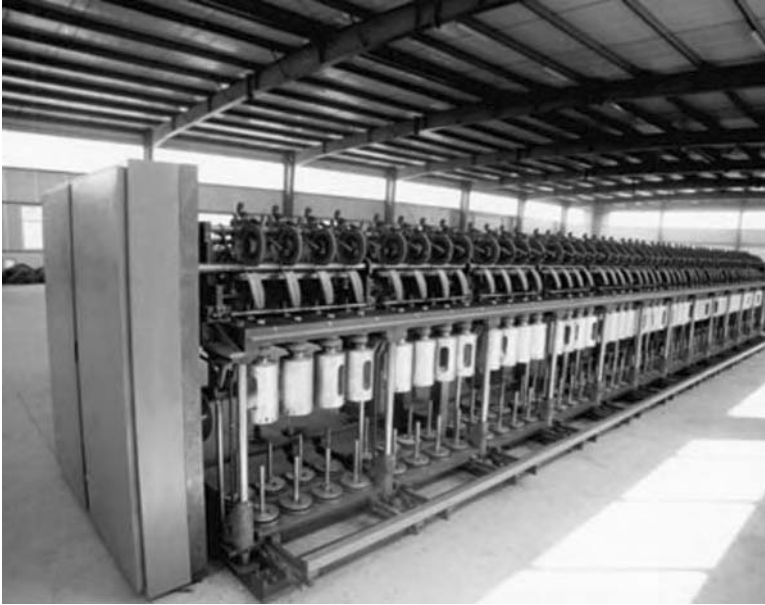
Figure 6.23 Vertical ring frame for sisal spinning.
