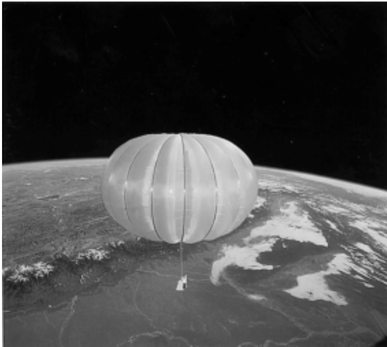
2.23 Balloon made of five-layered fabric with gas-barrier property (Teijin).
