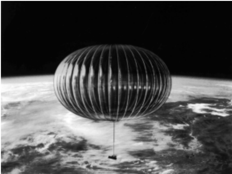
3.17 Pumpkin-shaped balloon for atmospheric observation (NASA).
