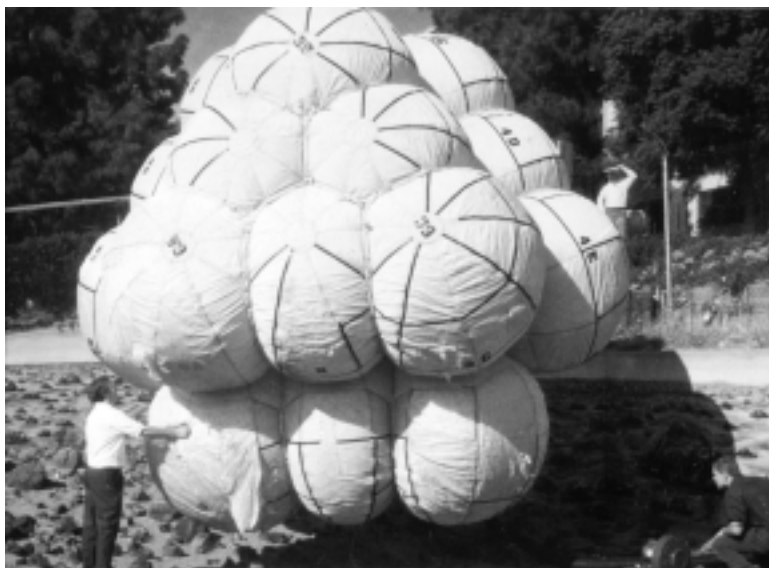
3.12 Space probe Mars Pathfinder covered with Vectran airbag (NASA).
