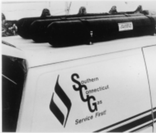
Natural gas cylinder on the roof
