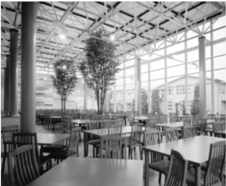
4.15 A view of Toray Ehime factory dining room where a solid truss roof made of CFRP was used for the first time (Toray).
