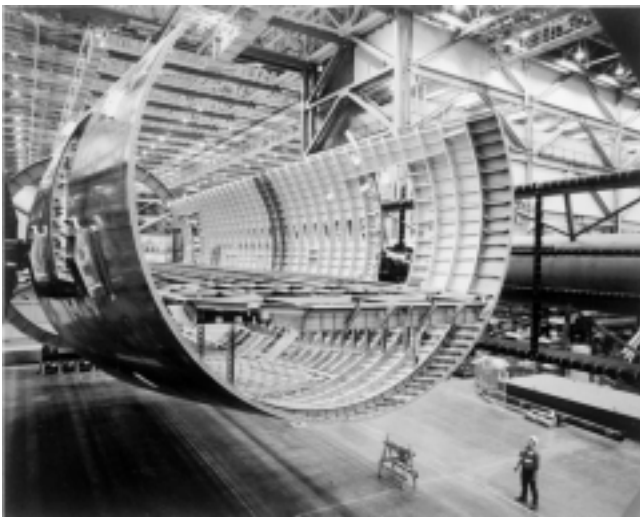
4.5 Carbon fiber composite material used for floor girder material of Boeing 777 (Boeing).
