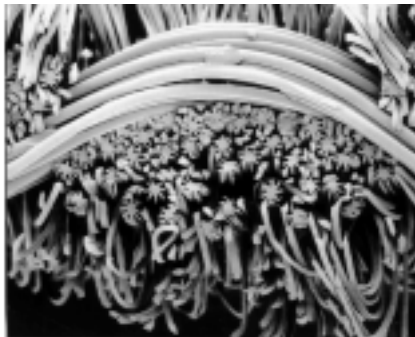
5.22 High multi-compact materials having minute structure and flexible touch ARTIROSA (Toray).
