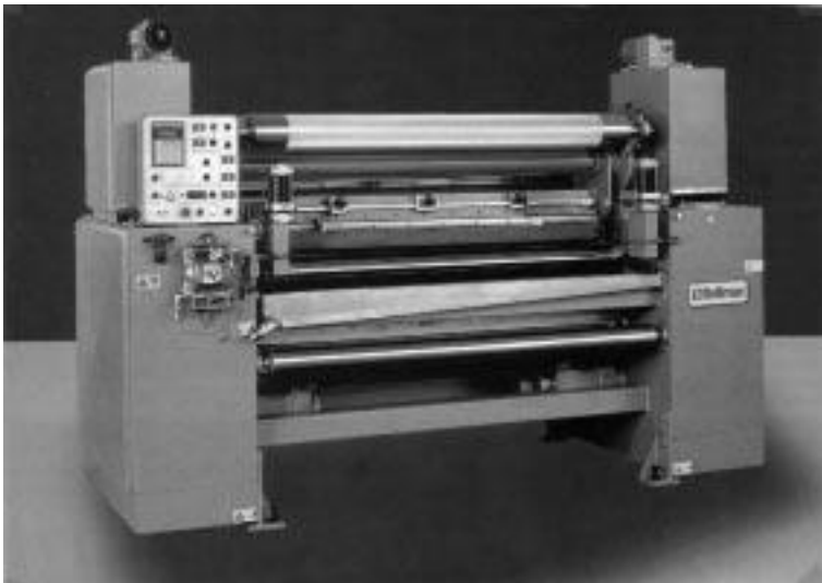
8.3 A multifunctional coating head for both direct and transfer coatings with either water-based or solvent-based resins. An engraved roller can also be used to apply resins on the same coating head. Source: Photograph reproduced by kind permission of Rollmac® International s.r.l. (Italy).
