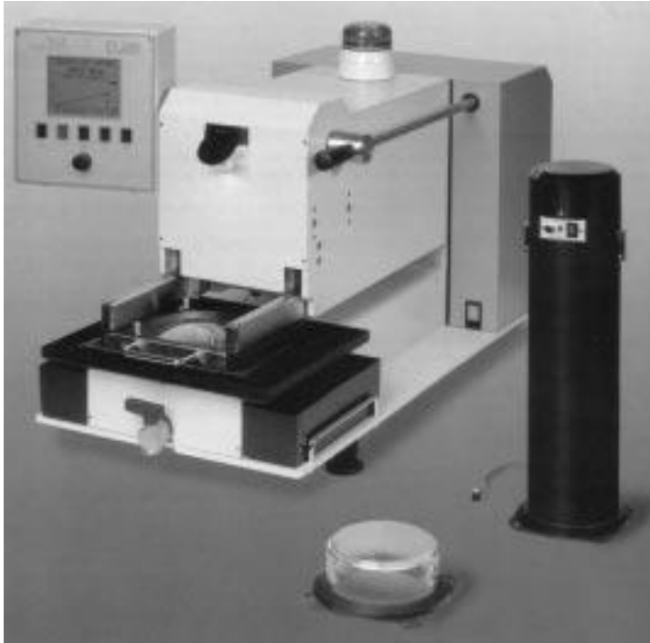
8.6 Modern hydrostatic head tester (FX 3000 Automatic Hydrostatic Head Tester 'Hydrotester 111' by Textest AG), for measuring water resistance of coated fabric. Water drops penetrating through the test fabric are automatically detected and so continuous operator attendance is not required during testing. Source: Photograph reproduced by kind permission of Textest AG of Zurich, Switzerland.
