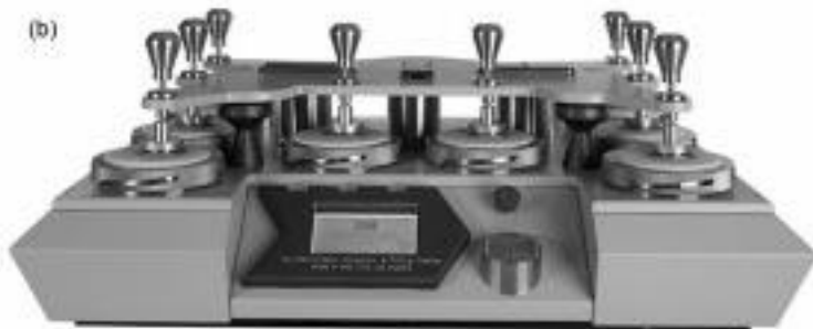
8.7 Martindale abrasion test apparatus. The photograph shows the advanced Nu-Martindale 864 model by James Heal and Co. Ltd of Halifax, England. The coated fabric is placed at the lower position of the test apparatus. This provides an abraded sample large enough for hydrostatic head testing after abrading. The 864 model, with the appropriate software, allows up to eight test samples being tested configured in two groups. Source: Photograph reproduced by kind permission of James Heal and Co. Ltd.
