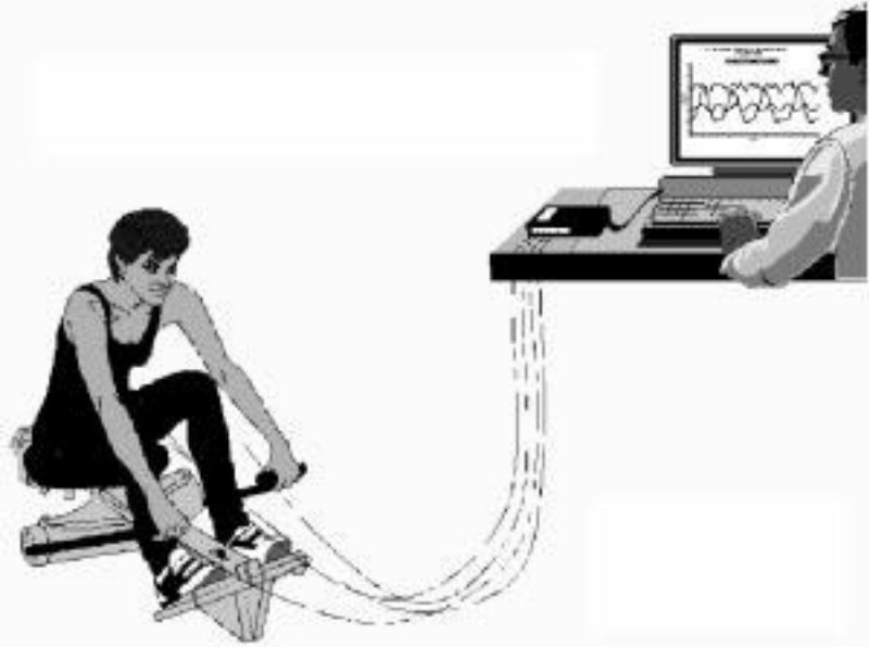
10.7 Schematic diagram of the dynamic force measurement device with sensors (Source: DuPont).
