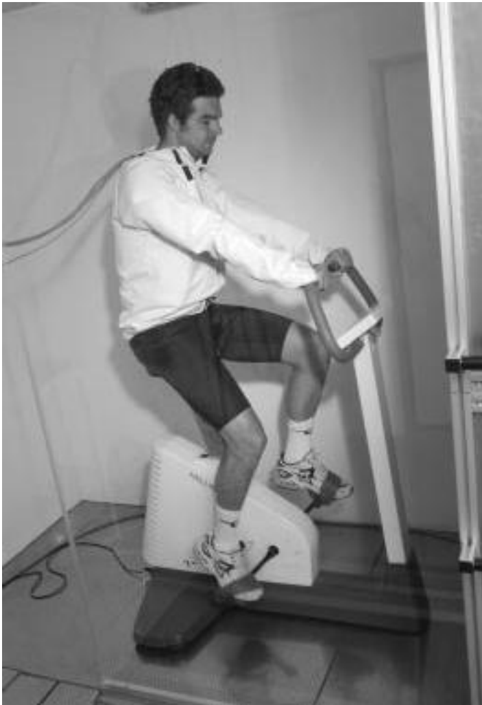
9.1 Wearer trial with a human subject testing bikewear in a climatic chamber.
